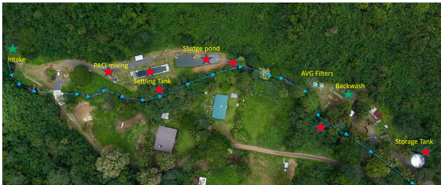
Figure 2 - Takuva'ine Water Treatment Plant where there is risk of PACI getting into the environment and where there is potential risk to the Plant from the environment.
