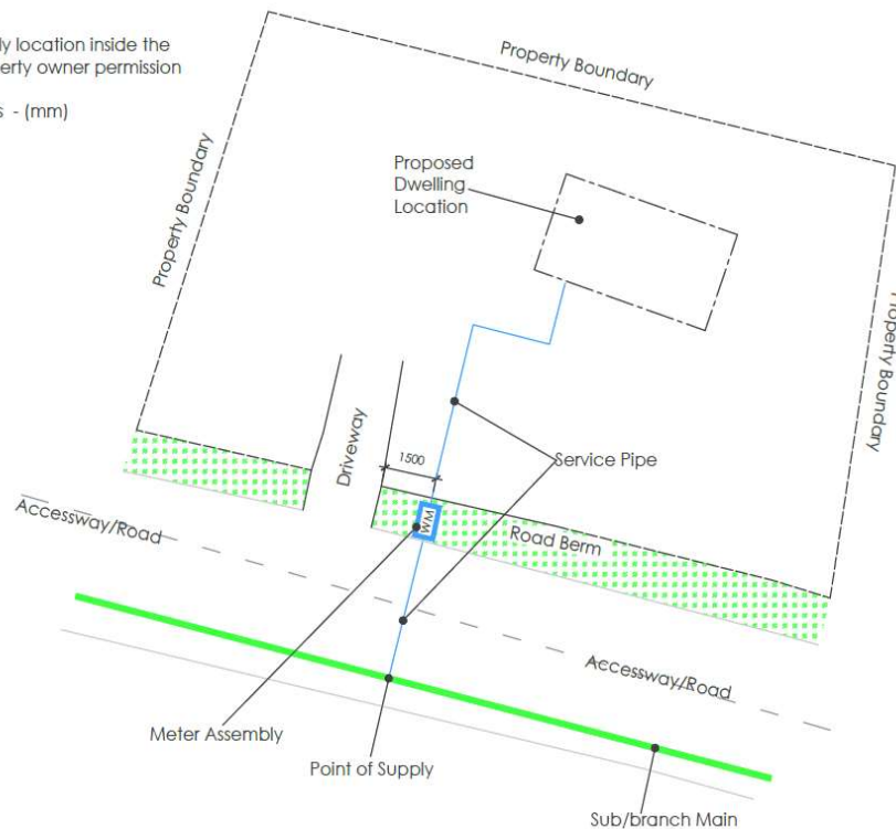
Figure 1: Typical layout of the water connection to the TTV network
